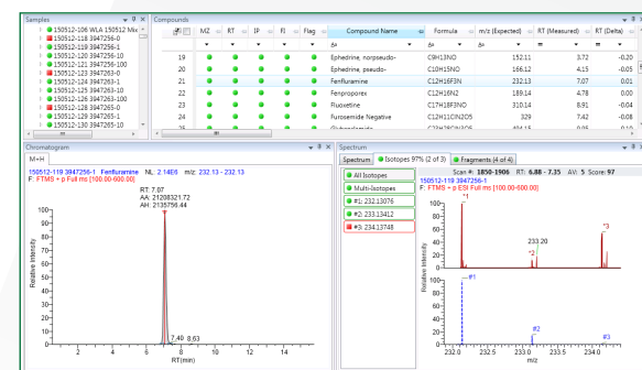
Figure 3. Workflow step for the determination of the isotopic pattern in a powder sample spiked with fenfluramine at 1ppm.
