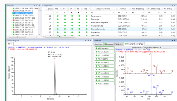
Figure 4. Workflow step for the evaluation of the fragments observed for homosibutramine in a powder sample spiked at 1ppm.
